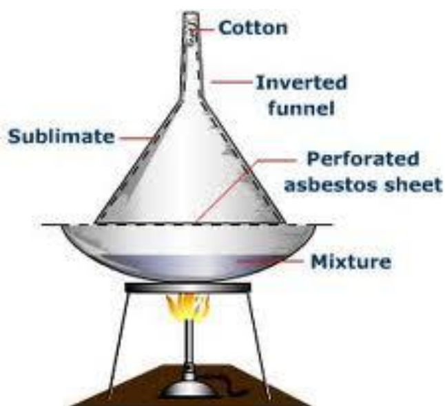
Figure 1.6: Sublimation set-up
