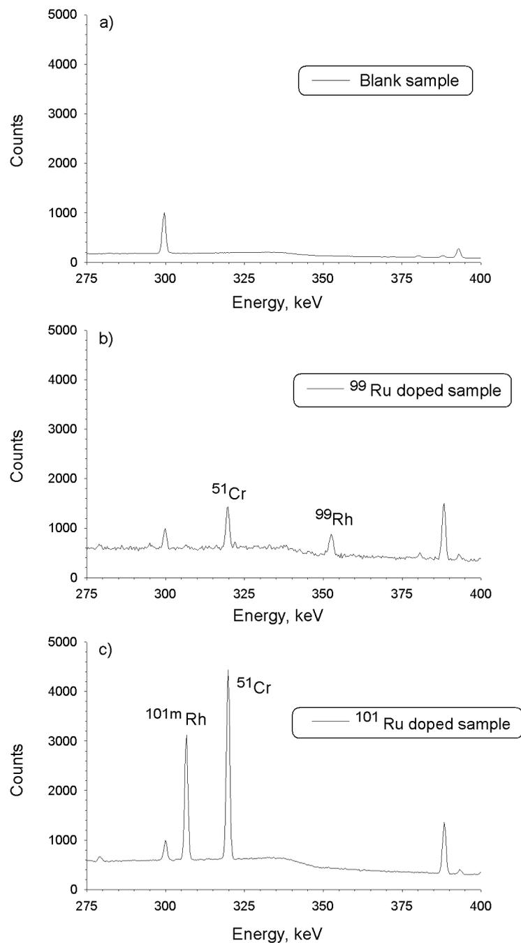
Fig. 1. Gamma-spectra after irradiation of a blank urine sample (a), of a urine sample containing  $^{99}\text{Ru}$  and  $^{51}\text{V}$  (b) and of a urine sample containing  $^{101}\text{Ru}$  and  $^{51}\text{V}$  (c)
