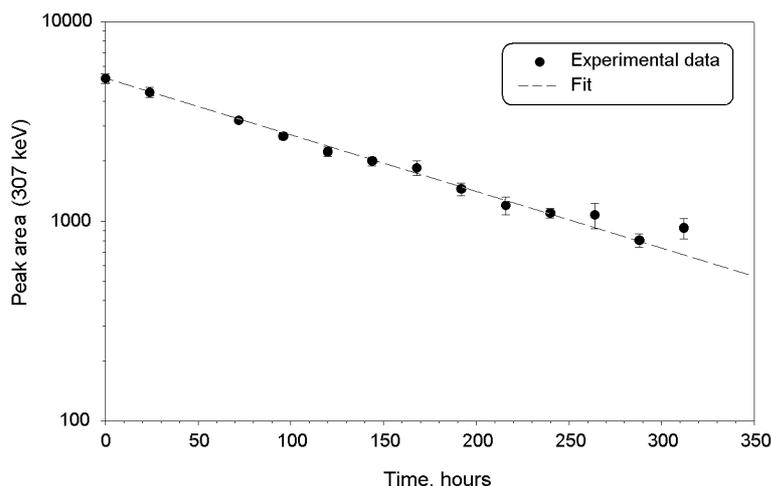
Fig. 2. Decay of the intensity of the gamma-line at 306.9 keV of  $^{99}\text{Rh}$  with time. The dashed line is a mono-exponential fit to the measured data
